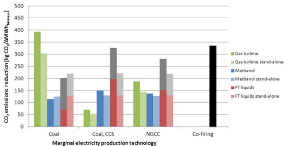
**Figure 3** Specific CO<sub>2</sub> emissions reduction of integrated and stand-alone energy mills for three different marginal electricity production technologies. The grey bar, on top of a red bar, indicates the reduction potential if CO<sub>2</sub> streams in the FT processes are captured and stored. The specific CO<sub>2</sub> emissions reduction potential of co-firing biomass in a coal power plant is shown for comparison.
