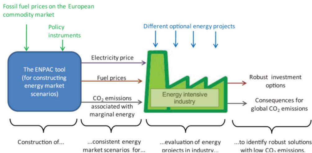
**Figure 1:** Overview of the purpose of energy market scenarios for evaluation of energy efficiency investments in energy intensive industry where the ENPAC tool is used to construct the scenarios.
