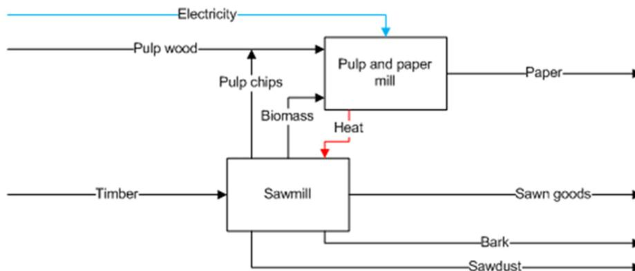
**Figure 2.** Energy and material flows of the combined TMP mill and sawmill. The biomass residues (bark, sawdust, cutter shavings) delivered from the sawmill to the TMP mill match the fuel demand of the steam boiler.
